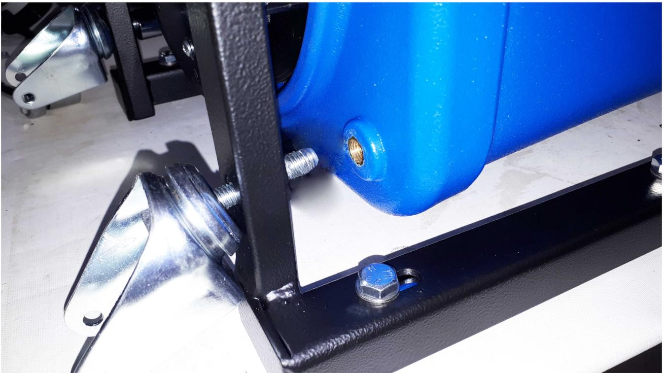
8. Hand thread the bolts back into the machine base, then using the 13 mm socket tighten until snug.
