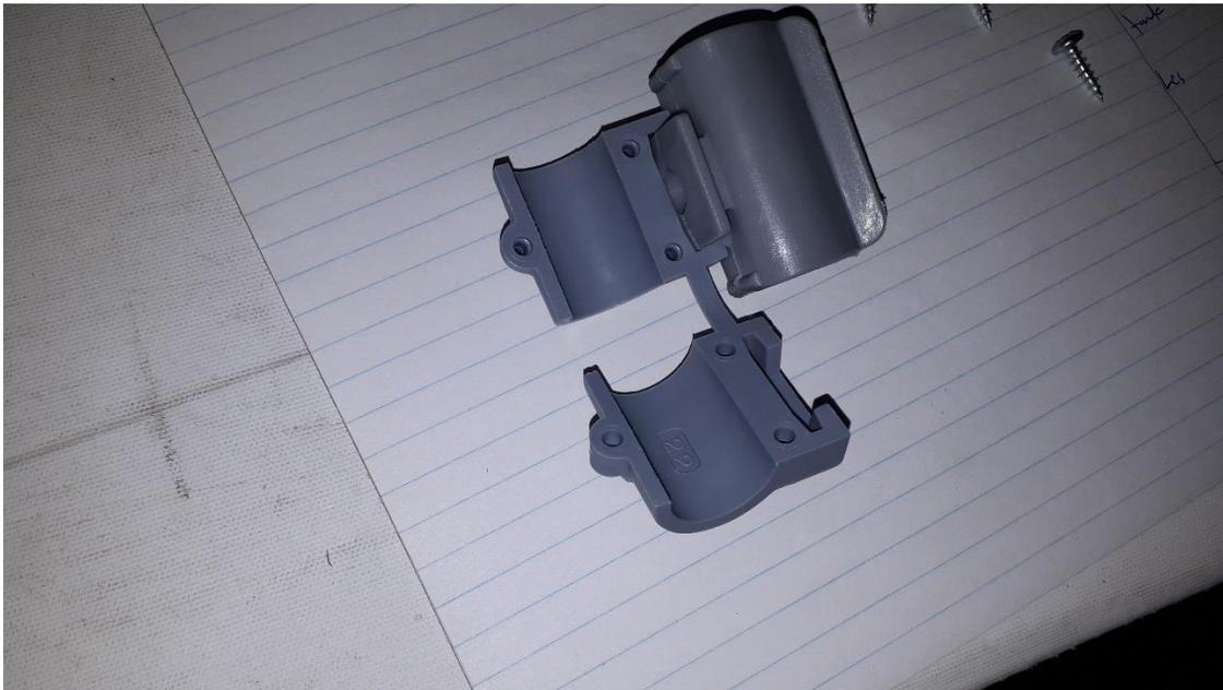
12. Attach grey holder to handle frame using three Phillips screws
