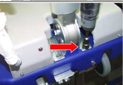
Connect the shock to the support. Connect the handle cable with the motor cable.
