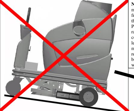
Note: If you must unload the machine in reverse, stand in front of the machine and pull the drive levers towards you. Push the machine down the ramp in reverse while continuing to hold the drive levers. Never drive the machine down a ramp in reverse. Also, ensure that the battery box is well secured when unloading in reverse.
