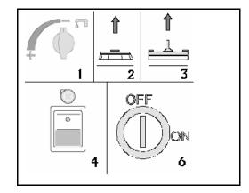
Take the hose off the hook, unscrew the drain plug and empty the recovery tank. To make this operation easier, keep the hose higher than the tank water level with one hand and with the other hand unscrew the knob and take off the cap. By slowly lowering the hose, the liquid will come out at the desired speed. Do this only when wearing protection gloves to prevent contact with dangerous solutions.
