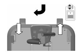
These pedals are meant to lock the direction of the front wheels to ensure straight drive when operating in forward or reverse gear.
