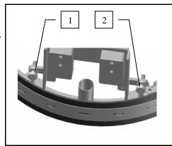
To release the squeegee from the machine, use the lever (1) and the squeegee is immediately released from its holder. Disconnect the suction hose and push it towards the inside of the machine to release the opposite side.
