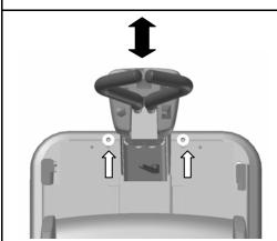
**NOTE**: the machine is fitted with a deadman microswitch. The machine does not works if the operator is not seated properly.
