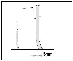
To adjust the squeegee blade down, just tilt back the squeegee body by turning the knobs counter-clockwise. To adjust the squeegee blade up, turn the knobs clock-wise. When adjustment is completed, thighen the lock-nut.
