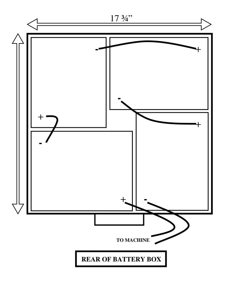
NOTE: Battery box will accept Trojan T125 Batteries (10 3/8" L x 7 3/8" W)
