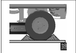
Push the machine backwards off of the skid using a ramp. Avoid hitting the brush head on the skid.
