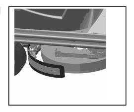
When operating the machine, the rear rubber should be slightly tilted back 5mm all along its length. you can use the squeegee on all 4 edges before replacing it with a new one.
