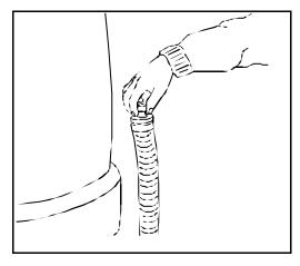
When the machine is not operating lift the squeegee to prevent rubber bars from losing their shape.
