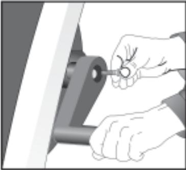
Put high pressure cleaner into upright position. Remove the screw from the brass element. Put the crank on the hexagon and fasten with the screw.
