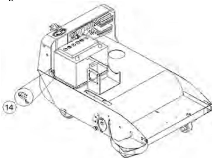
6. Once the cover is removed, you must connect the battery cables to the battery. When connecting the battery terminals, do not reverse the polarity. Ensure that the red wire goes to the + terminal and the black wire goes to the - terminal on the battery.
