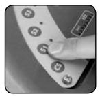
Settings can be stored using one of the three pre-set store buttons (S1 / S2 / S3). Once settings are entered (chemical dose, brush speed and water-flow), press and hold one of the three pre-set store buttons, a light will flash then remain constant; your settings are now saved. This facility can be re-set as often as you wish by simply following the steps above.
