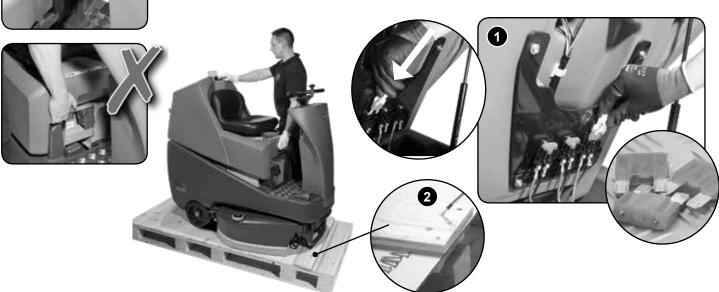
Lift top tank assembly to reveal battery compartment.
