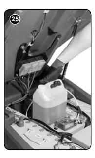
To fill the chemical dosing bottle, first lift up the waste-water tank (Fig.23), remove the dosing bottle, unscrew the bottle cap (Fig.24) and fill with appropriate cleaning chemical. Replace bottle cap, refit dosing bottle (Fig.25) and carefully lower waste-water tank.
