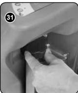
Turn it anti-clockwise to decrease load on the brushes and clockwise to increase load / pressure on the brushes (see Fig.31).
