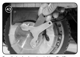
Once the key has been inserted (see Fig.43) the motor brake will be fully disengaged.
