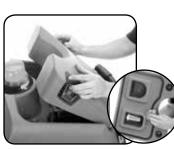
Before removing separator, first pull-off connected hoses. Whilst pressing in the separator toggles, remove hood and rinse using clean-water. The hood also has a sealing-rubber which should be examined at every clean-down.
