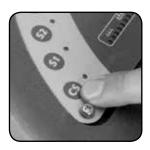
Cleaning Speed setting (CS). When this button is activated the speed is restricted to 3.5 km/h maximum even with the accelerator pedal fully depressed. This is ideal for long cleaning periods. Once this pre-set button is switched-off, the machine will operate at up to a maximum speed of 7.0km/hr.
