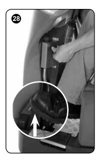
After preparing the floor (see previous section), we are now ready to set the controls to suit the cleaning conditions. Before any settings can be applied, ensure the brush deck is lowered.
