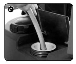
To fill the clean-water tank, lift the cover flap (Fig.19) to expose the filler cap. Unscrew the filler cap (Fig.20) and fill the tank using a hose (Fig.21) or preferred method.
