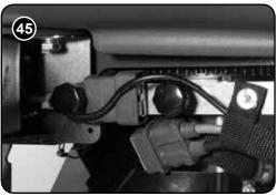
Pull the power conector block apart and refit the two retaing knobs.
