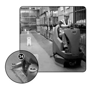
To operate, select forward or reverse, press the accelerator pedal. Vacuum pick-up, water-flow and chemical-dose will turn on automatically and the machine will move forward.
