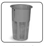
The secondary clean-water tank filter is located to the rear of the battery compartment, and should be checked at regular intervals. Lift white plug and remove the filter, rinse and refit. Ensure tank has been emptied and care is taken when working in the vicinity of batteries.
