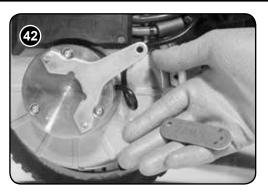
Your start-up kit includes a brake drive disengage key (329945, see Fig.42) which can be inserted between the brake arm and drive housing (see Fig.43).
