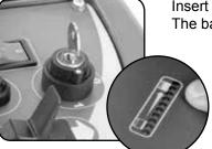
Insert key into main control (on / off) and turn quarter-turn clockwise to position (1) 'ON'. The battery charge level meter will illuminate.
